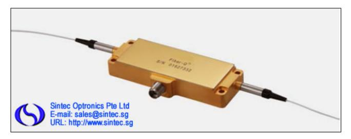
The STG-T-M080-0.5C8J-3-F2P acousto-optic modulator is designed for use as an 80 MHz frequency shifter for heterodyne interferometry or as an intensity modulator.
