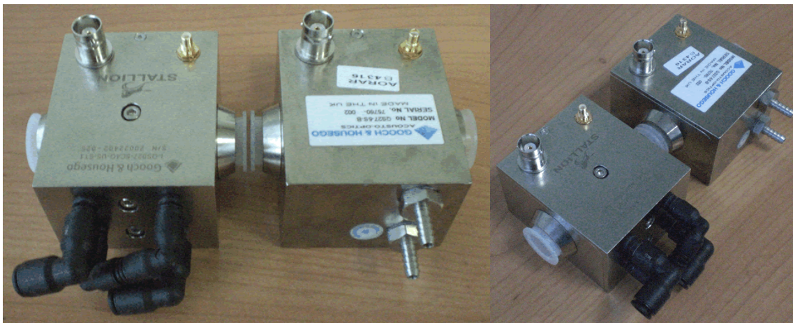
Comparison between Stallion and old Q-switches. The main difference of the outlooks is water connector.
