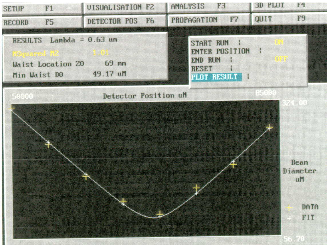
Figure 4.5 Focused beam propagation parameters given by the beam diagnostic system
