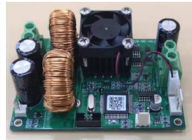
temp. control board
