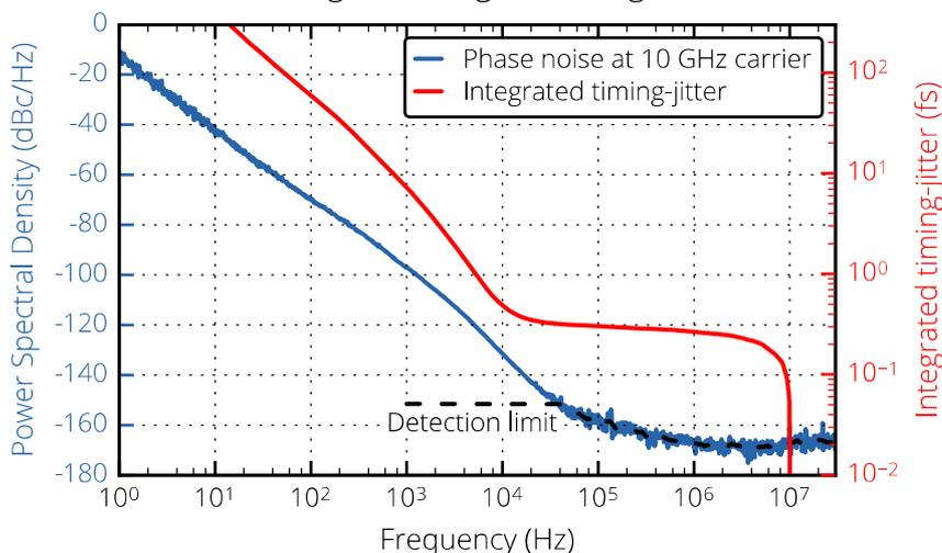
Figure 2 — Phase noise (left/blue) and timing-jitter (right/red) of the MENHIR-1550 laser, measured on the 10<sup>th</sup> harmonic signal (10 GHz). The black dashed-line represents the detection limit of the characterization setup and does not represent the intrinsic limit of the laser.
