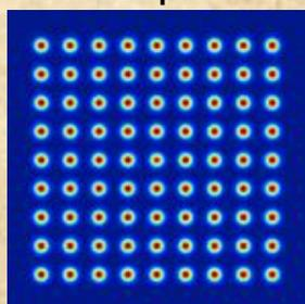
Such applications require precise microscopic holes of a desired pattern with equal distances. This is the beam-splitter DOE are the obvious solution.
