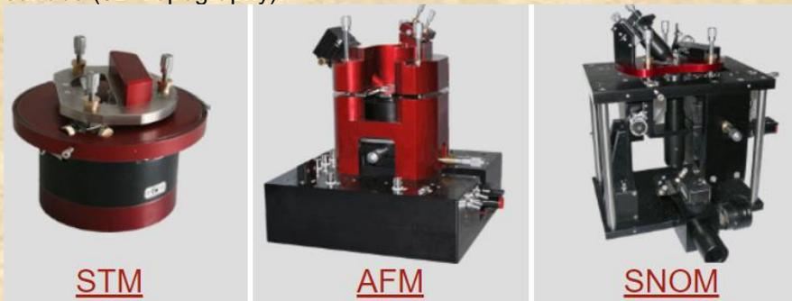
It is possible to acquire different physical properties (electric, magnetic, optical, ...) of the sample, obtaining different images of the sample, using different type of probe. STM, AFM and SNOM represent different type of SPM Microscopes that are characterized by a different measuring probe.
