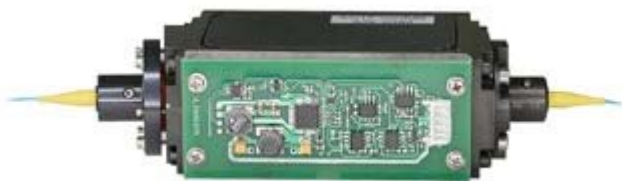
Our acousto-optical tunable filter with fiber-optic delivering system is at the heart of the Broadsweeper.
